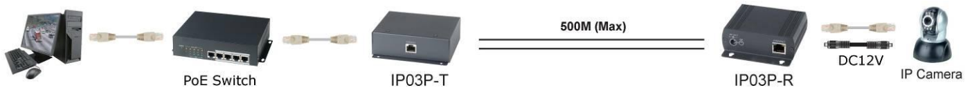
IP03PT with POE switch power input to IP03R and Non-POE IP camera.
