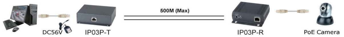
IP03PT with DC 48/56V Power adapter power input to IP03R and POE camera
